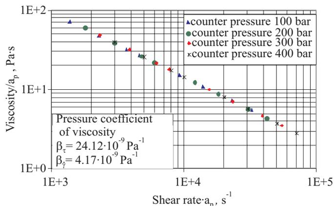
Fig. 5. Pressure invariant master curve of polypropylene PP HG313MO, shifted to the reference pressure of  $2 \cdot 10^7 \text{ Pa}$  (200 bar) at a temperature of 210 °C
