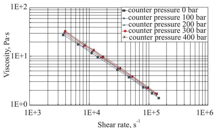
Fig. 4. Pressure dependency of polypropylene PP HG313MO, measured at a temperature of 210 °C and 5 counter pressure levels
