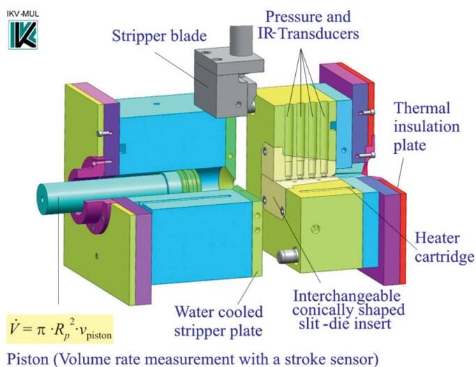
Fig. 1. Rheological injection mould
