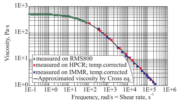
Fig. 3. Viscosity curve of polypropylene PP HG313MO at a temperature of 210 °C, measured using standard rheometers (RMS800 or HPCR) and the injection moulding machine rheometer (IMMR), cross approximation [9]
