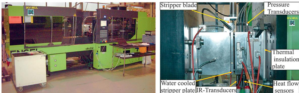
Fig. 2. Injection moulding machine with rheological injection mould
