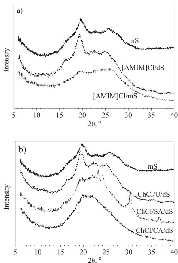
Fig. 2. Comparison of XRD diffractograms of native starch (*mS*) with that obtained for residues after thermoplasticization in rheometric test conditions of ILs/starch systems with mass ratio 30:100: a) [AMIM]Cl and dry or moist starch, b) based on dry starch with ChCl itself and deep eutectic mixtures of ChCl with urea (ChCl/U 1:2 mol/mol), citric acid (ChCl 2:1 mol/mol) and succinic acid (ChCl/SA 1:1 mol/mol)
