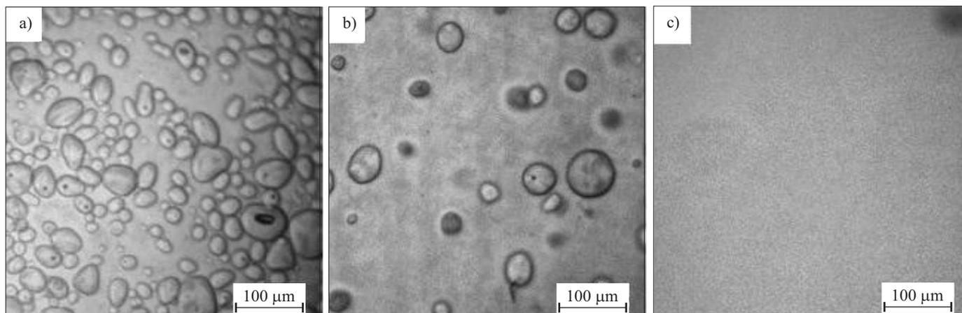
Fig. 3. LSM micrographs for 5 wt. % dry potato starch in ChCl/U eutectic mixture after 1 h solubility tests at: a) 80 °C, b) 100 °C, c) 118 °C
