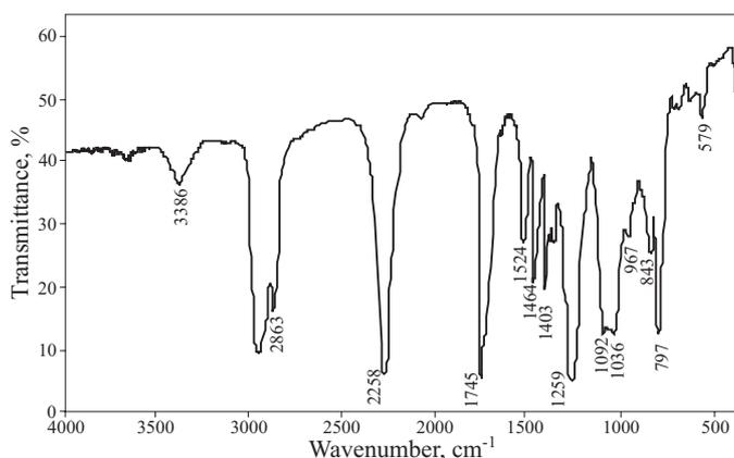
*Fig. 4.* FT-IR spectrum of the urethane prepolymer based on co-MD4 and IPDI (NCO:OH = 3:1)
