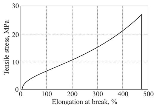
Fig. 6. Stress-strain curve of PUU elastomer based on co-MD3
