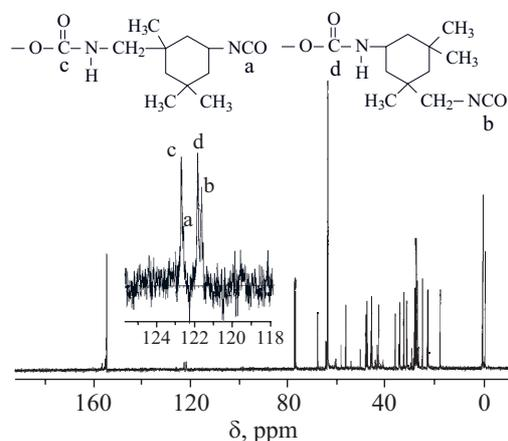
*Fig. 5.*  $^{13}\text{C}$  NMR (400 MHz,  $\text{CDCl}_3$ ) spectrum of the urethane prepolymer based on co-MD4 and IPDI (NCO:OH = 3:1)
