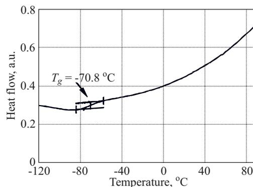
Fig. 7. The DSC thermogram of PUU based on co-MD3
