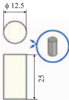
Fig. 1. The specimen used for mechanical properties of adhesive composite determination
