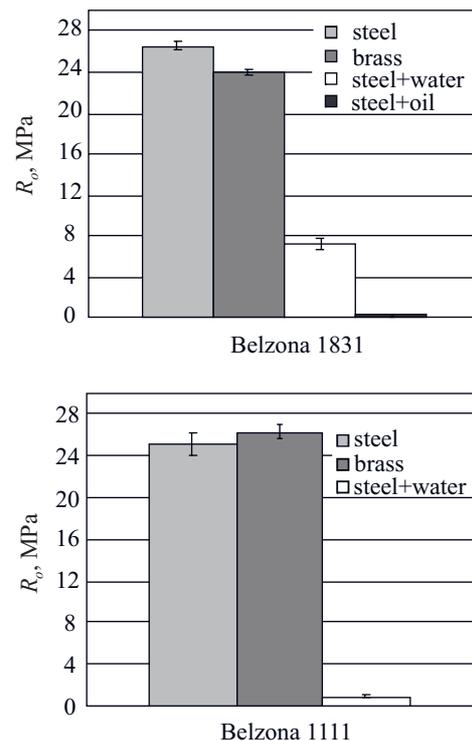
Fig. 6. Tensile strength of Belzona 1831 and Belzona 1111 adhesive composite for steel, brass, wet steel, and covered with oil steel specimens
