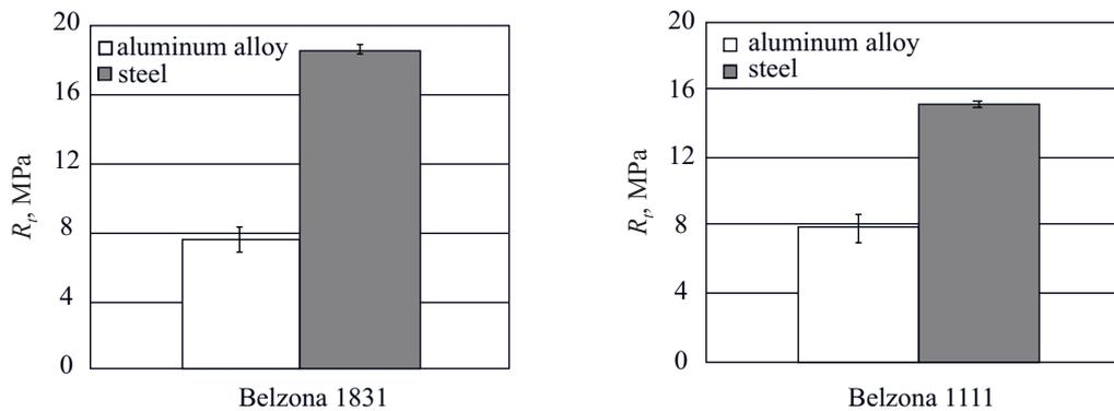
Fig. 7. Shear strength of Belzona 1831 adhesive composite for aluminium and steel specimens
