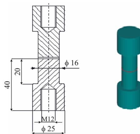
Fig. 2. The specimen used to determine strength properties of adhesive composite
