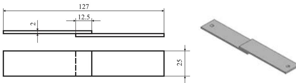
Fig. 3. The specimen used to determine utilitarian properties of adhesive composite
