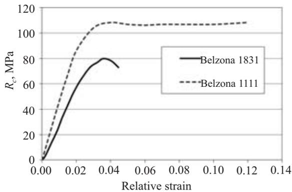
Fig. 4. Exemplary compression curves obtained for Belzona 1831 and Belzona 1111 adhesive composites
