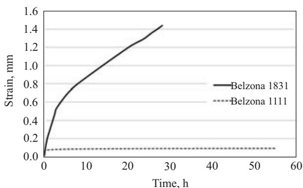
Fig. 5. Creep curves obtained for Belzona 1831 and Belzona 1111 adhesive composite at the temperature of 20 °C with load causing normal stresses of 30 MPa in the tested specimen
