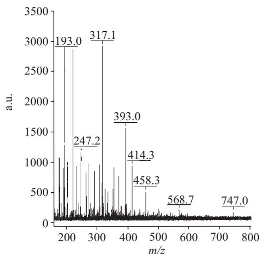
Fig. 3. MALDI ToF spectrum of the reaction product of mixture BHEOD and boric acid with EC 1:10 in the presence of 0.09 mole K<sub>2</sub>CO<sub>3</sub>/mole BHEOD at 160 °C
