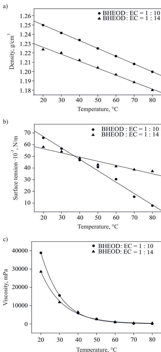
Fig. 6. Physical properties of products of reactions of mixture BHEOD and boric acid with EC as a function of temperature
