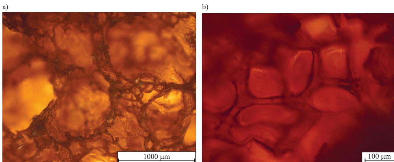
Fig. 7. Morphology of the foam derived from polyols obtained as a product of reaction of mixture of BHEOD and boric acid and: a) 10-, b) 14-molar excess of EC, magnification: a) 2.5×, b) 10×
