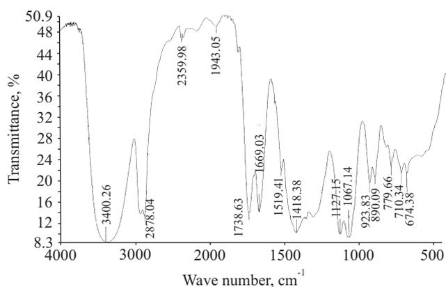
Fig. 5. IR spectrum of the reaction product of mixture BHEOD and boric acid with EC 1:14 in the presence of 0.12 mole  $K_2CO_3$ /mole BHEOD at 160 °C
