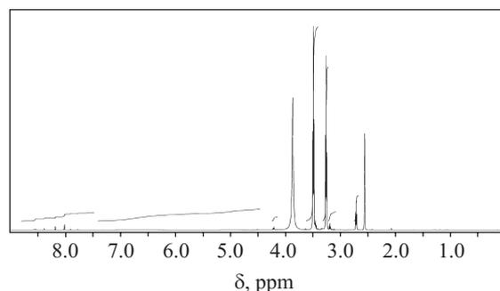
Fig. 2.  $^1\text{H}$  NMR spectrum of the reaction product of BHEOD with boric acid with the addition of  $\text{D}_2\text{O}$
