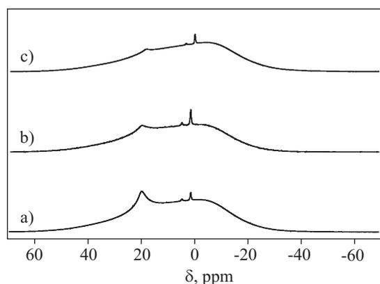
Fig. 1.  $^{11}\text{B}$  NMR spectra of the reaction product of BHEOD with boric acid taken after: a) 5, b) 15, c) 25 minutes of reaction
