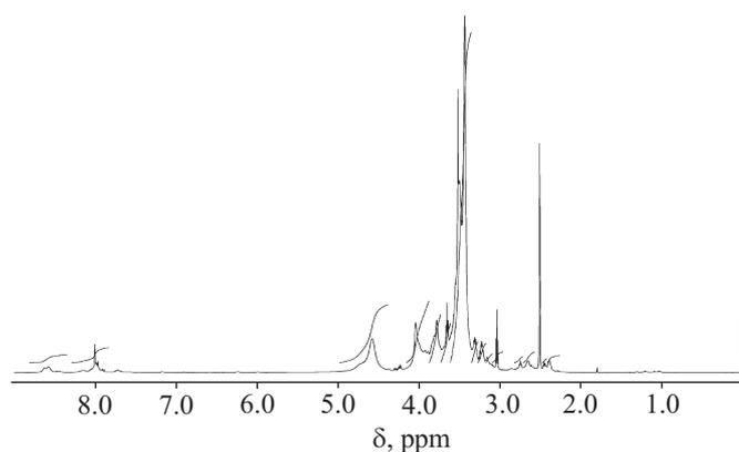
Fig. 4. <sup>1</sup>H NMR spectrum of the reaction product of mixture BHEOD and boric acid with EC 1:14 in the presence of 0.12 mole K<sub>2</sub>CO<sub>3</sub>/mole BHEOD at 160 °C
