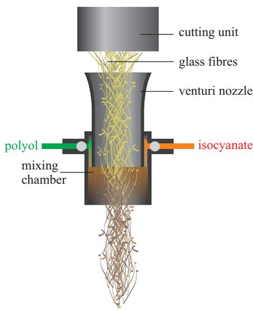
Fig. 1. Scheme of the LFI mixing head
