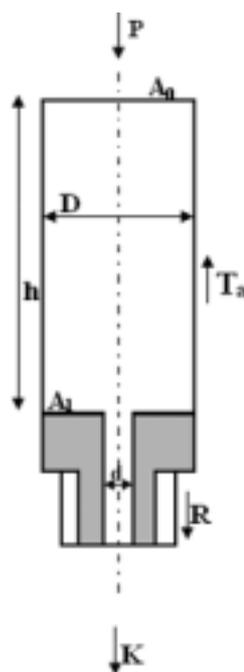
Fig. 2. Loading system in the rheometer during material flow:  $P$  — set load,  $A_0$  — cross-section area of cylinder,  $A_1$  — upper plane of the die,  $R$  — value measured by the force sensor,  $T_a$  — adhesive friction,  $K$  — flow resistance in capillary tube,  $D$  — diameter of cylinder,  $d$  — capillary tube diameter,  $h$  — height of polymer column level in the cylinder
