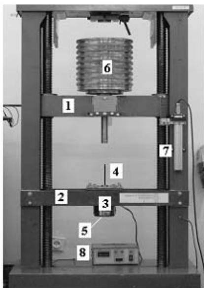
Fig. 1. Capillary piston rheometer: 1 — moving toolbar, 2 — stationary toolbar, 3 — cylinder with heating system, 4 — piston, 5 — force sensor, 6 — piston load, 7 — linear displacement transducer, 8 — temperature control system
