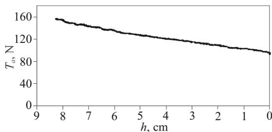
Fig. 4. Dependence of adhesive friction ( $T_a$ ) as a function of height of polymer column level in cylinder of the rheometer ( $h$ )
