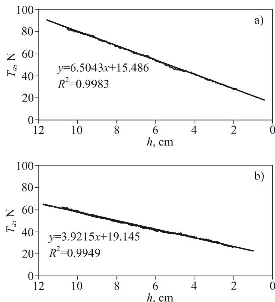
Fig. 5. Dependence of adhesive friction ( $T_a$ ) as a function of height of P-PVC level in cylinder of the rheometer ( $h$ ) at temp. 140 °C for different imposed load  $P$ : a) 400 N, b) 300 N
