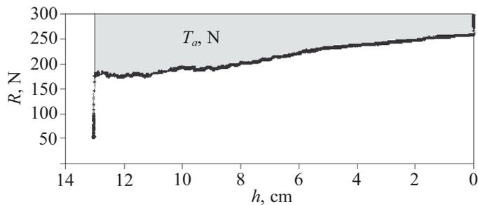
Fig. 3. Dependence of load  $R$  as a function of height of polymer column level in cylinder of the rheometer ( $h$ ) recorded at temp. 130 °C
