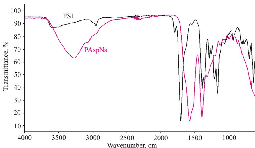
Fig. 1. FT-IR spectrum of polysuccinimide (PSI) and poly(sodium aspartate) (PAspNa)
