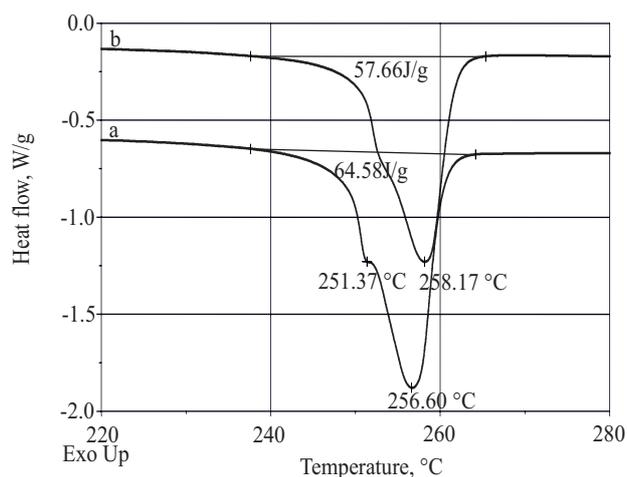
Fig. 6. DSC curves of flame retardant PET fibers modified with 15 % Roflam E in bath of temperature 130 °C: a) after 5 years of ageing in atmospheric conditions, b) directly after the fabrication; heating rate 10 °C/min, atmosphere N<sub>2</sub>, flow 40 cm<sup>3</sup>/min; analysis of the melting region
