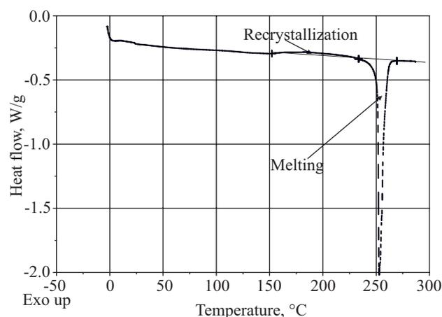
**Fig. 1. Shape of exemplary DSC curve (sample modified in 130 °C, Roflam E content 5 %) of studied PET flame retardant fibers during the heating (10 deg/min) in nitrogen (flow 40 cm<sup>3</sup>/min) from 0 to 280 °C**
