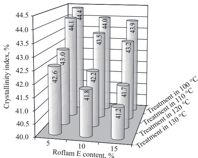
Fig. 2. Changes of crystallinity index of modified flame retardant PET fibers, evaluated on the basis of DSC measurements, as a function of Roflam E content and the temperature of modifying bath
