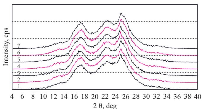
Fig. 3. WAXS patterns of PET fibers modified with different contents of Roflam E: 1 – PET + 5 % Roflam E/100 °C, 2 – PET + 15 % Roflam E/100 °C, 3 – PET + 5 % Roflam E/120 °C, 4 – PET + 15 % Roflam E/120 °C, 5 – PET + 5 % Roflam E/130 °C, 6 – PET + 15 % Roflam E/130 °C, 7 – PET + 30 % Roflam E/130 °C
