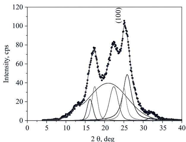
Fig. 4. Exemplary WAXS curve for a sample of fibers modified with Roflam E (15 %) in the temperature of 130 °C resolved for individual diffraction peaks
