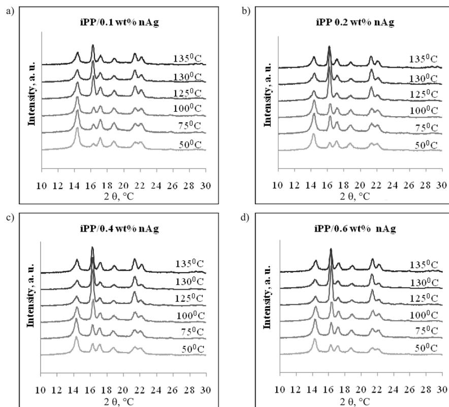
Fig. 4. WAXS patterns of iPP/nAg nanocomposites obtained in isothermal conditions containing: a) 0.1 wt % nAg, b) 0.2 wt % nAg, c) 0.4 wt % nAg, d) 0.6 wt % nAg
