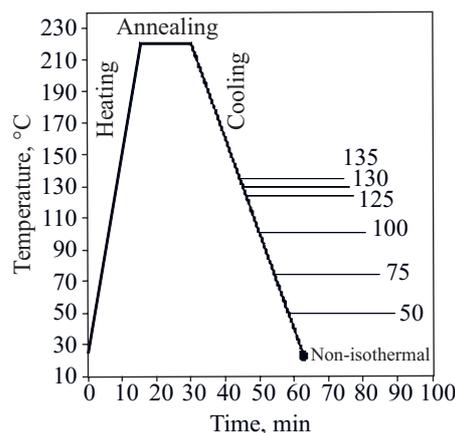
Fig. 1. Temperature program used in the recrystallization of nanocomposites of polypropylene with silver nanoparticles
