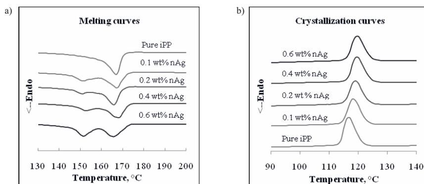
Fig. 5. Melting (a) and crystallization (b) curves of the pure iPP and composites obtained in non-isothermal conditions
