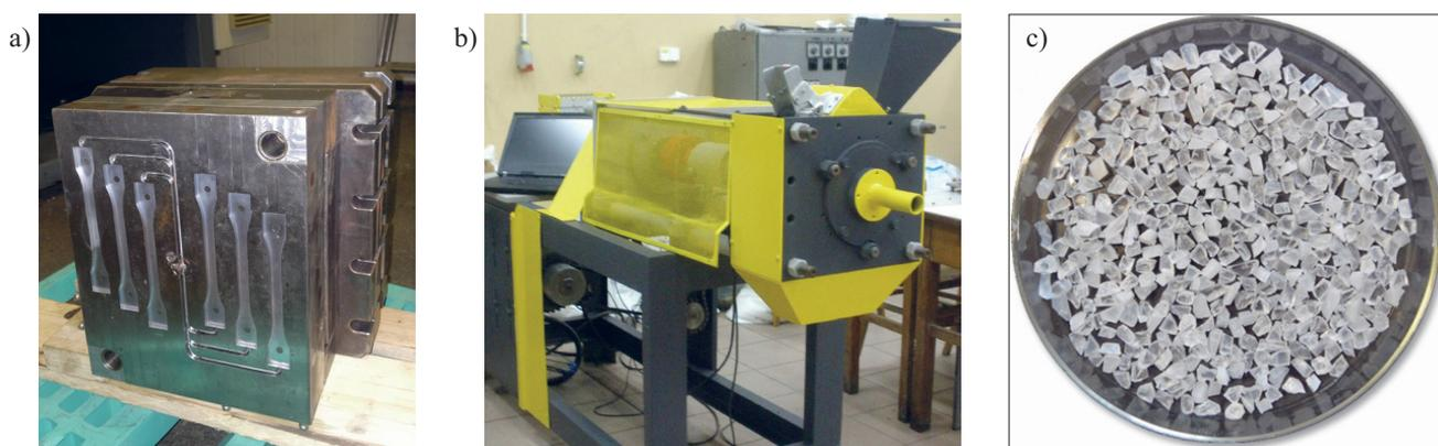
Fig. 1. Photographs of: a) experimental injection mold, b) cutting and grinding stand for polypropylene porous moldings, c) ground foamed samples
