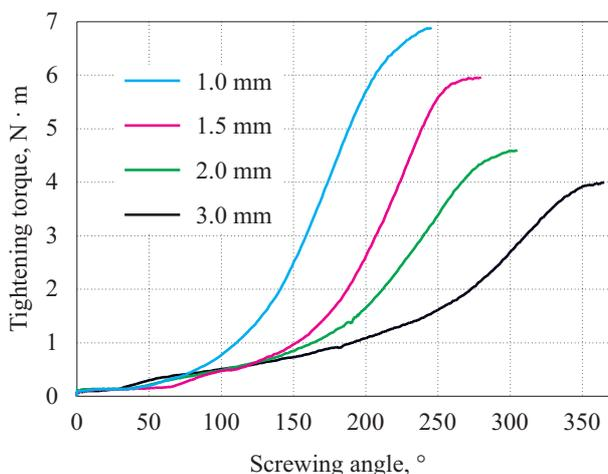
Fig. 3. The influence of the screwing angle of the screw cap on the tightening torque for different thicknesses of a sealing insert (exemplary courses)
