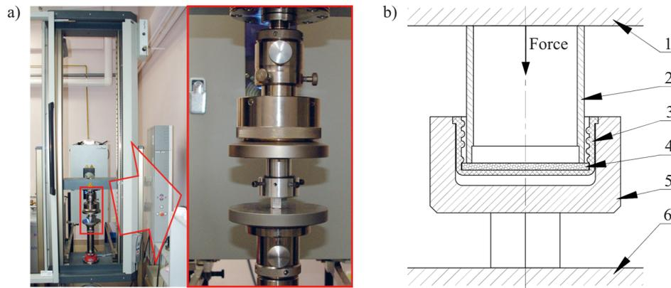
Fig. 2. Compression testing on a stress-strain machine Zwick Z030: a) testing on a stress-strain machine (the magnified image shows test stand elements), b) scheme showing invisible elements and method of testing [1 – movable compressing plate (arrow-direction of plate movement), 2 – bushing (container neck), 3 – polymer screw cap, 4 – tested sealing insert, 5 – holder of screw cap, 6 – immovable compressing plate]
