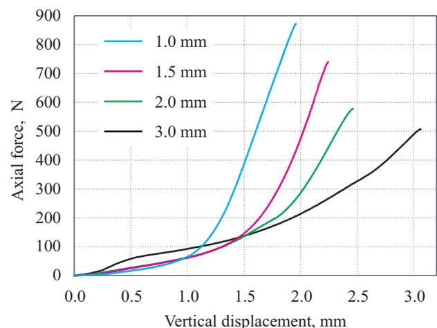
Fig. 4. The influence of vertical displacement during moving between the threaded connection elements on the axial force for different thicknesses of sealing insert (exemplary courses)
