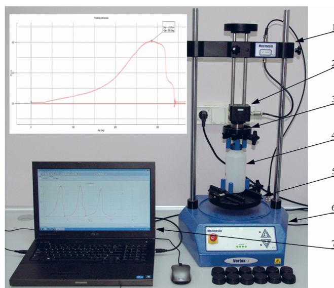
**Fig. 1. The laboratory stand for testing of threaded connections of a packaging (an example of a recorded course of tightening torque of a screw cap shown in magnification): 1 – stand frame, 2 – torque sensor, 3 – fixed holder, 4 – tested threaded connection, 5 – movable holder, 6 – stand base, 7 – control computer**
