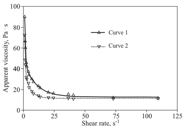
Fig. 1. Changes in apparent viscosity of EPBP1K-3.0 composite at increasing (curve 1) and decreasing (curve 2) shear rate
