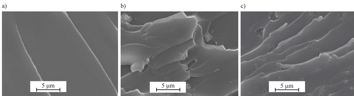
Fig. 3. SEM microphotographs of brittle fracture surfaces of: a) unfilled EP, b) EPBP1K-3.0, c) EPBP1K-4.5
