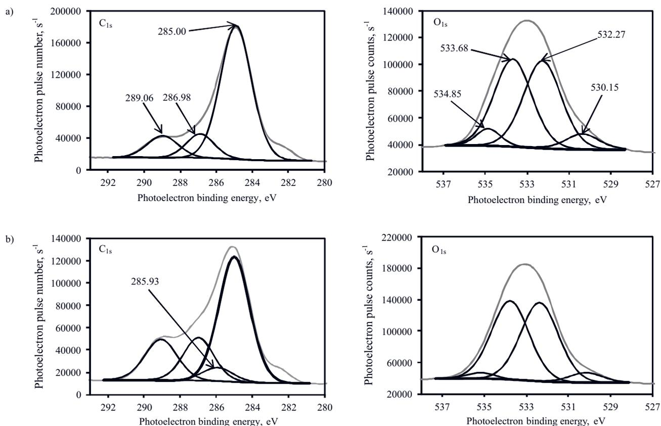
Fig. 2. XPS detailed  $C_{1s}$  and  $O_{1s}$  spectra of the: a) unmodified PLA, b) P60\_1000 specimens
