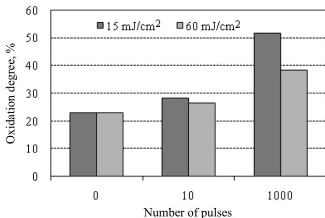
Fig. 3. Effect of the number of pulses on PLA surface layer oxidation
