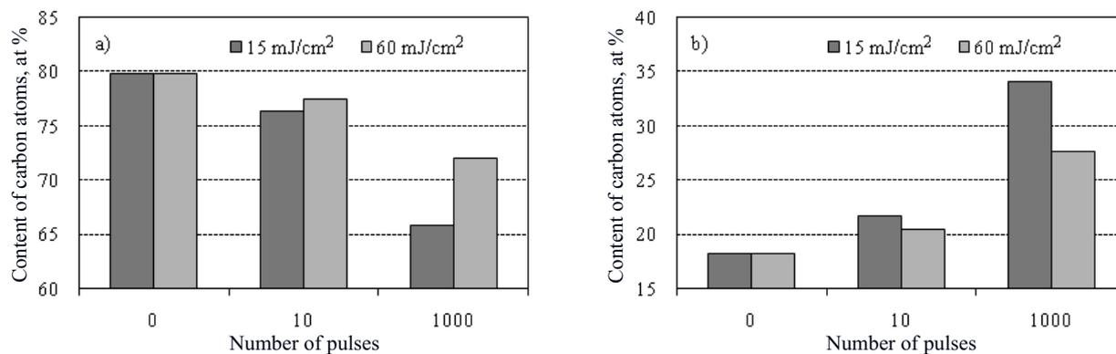
Fig. 1. Effect of the number of pulses on the contents in PLA surface layer of: a) carbon ( $C_{1s}$ ), b) oxygen ( $O_{1s}$ )
