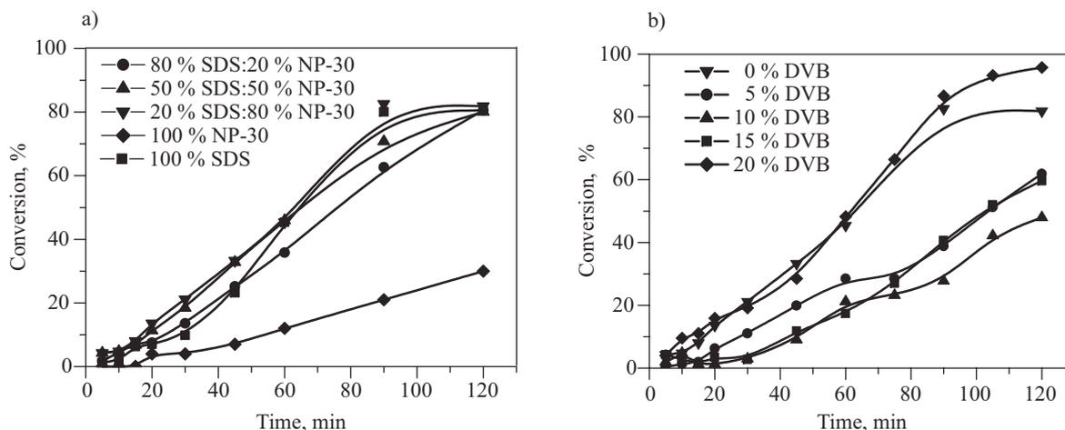
**Fig. 1. Conversion-time curves for emulsion polymerization of styrene at 80 °C: a) using different ratios of emulsifiers, b) at emulsifier ratio (20 % SDS: 80 % NP-30) with DVB as a crosslinking agent**
