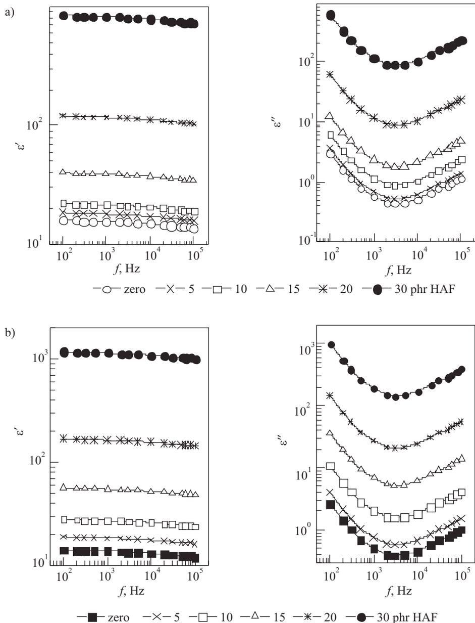
Fig. 10. The permittivity  $\epsilon'$  and dielectric loss  $\epsilon''$  versus the applied frequency  $f$  for: a) NBR composites without crosslinked PS, b) NBR composites with 5 phr crosslinked PS loaded with different contents of HAF
