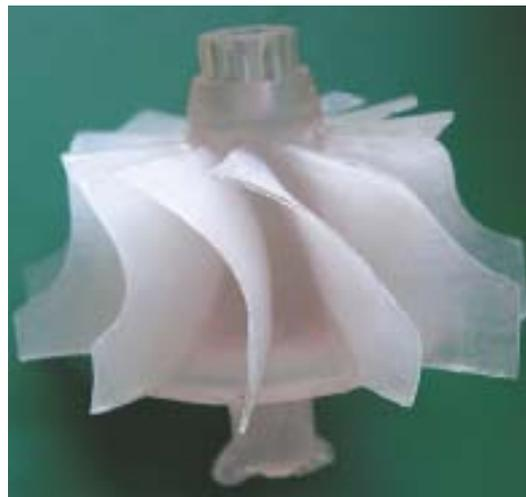
Fig. 3. Appearance of an impeller obtained from composite based on Polimal® 109-32 RPyK with 1.5 phr of BS modified with QAS2
