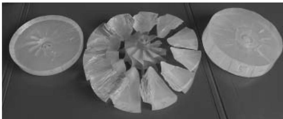
Fig. 1. Appearance of silicon mold matrix used for casting of models made of composites tested
