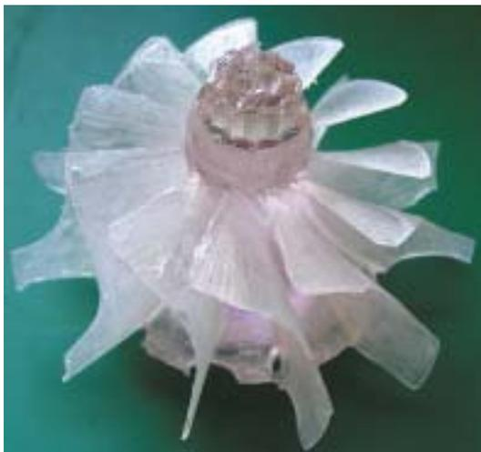
Fig. 2. Appearance of an impeller obtained from composite based on Polimal® 109-32 RPyK with 3 phr of BS modified with QAS2
