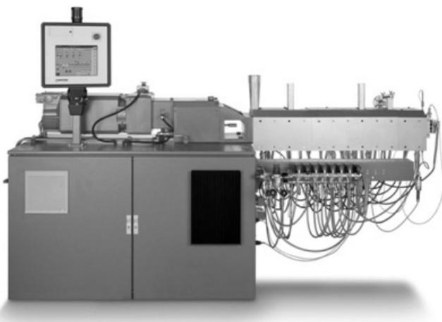
Fig. 3. Extruder Coperion ZSK 26 Mc used for experimental
