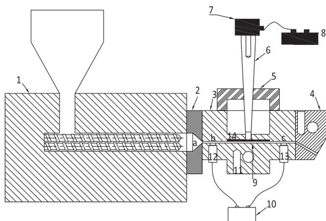
Fig. 1. The scheme of the designed extrusion head: 1 – extruder, 2 – coupling head, 3 – upper split case, 4 – die, 5 – sonotrode-transducer support, 6 – sonotrode, 7 – transducer, 8 – ultrasonic generator, 9 – rectangular profile channel, 10 – measurement chain, 11 – lower split case, 12 – sensor located before ultrasounds application area (b), 13 – sensor located after ultrasounds application area (c), 14 – separation sheet, a – location of the extrusion pressure sensor
