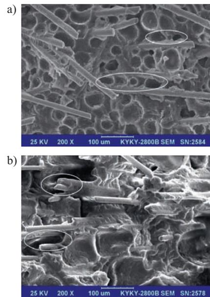
Fig. 5. SEM micrographs of the foam structure for: a) PP/GF/SiO<sub>2</sub>, b) PP/GF
