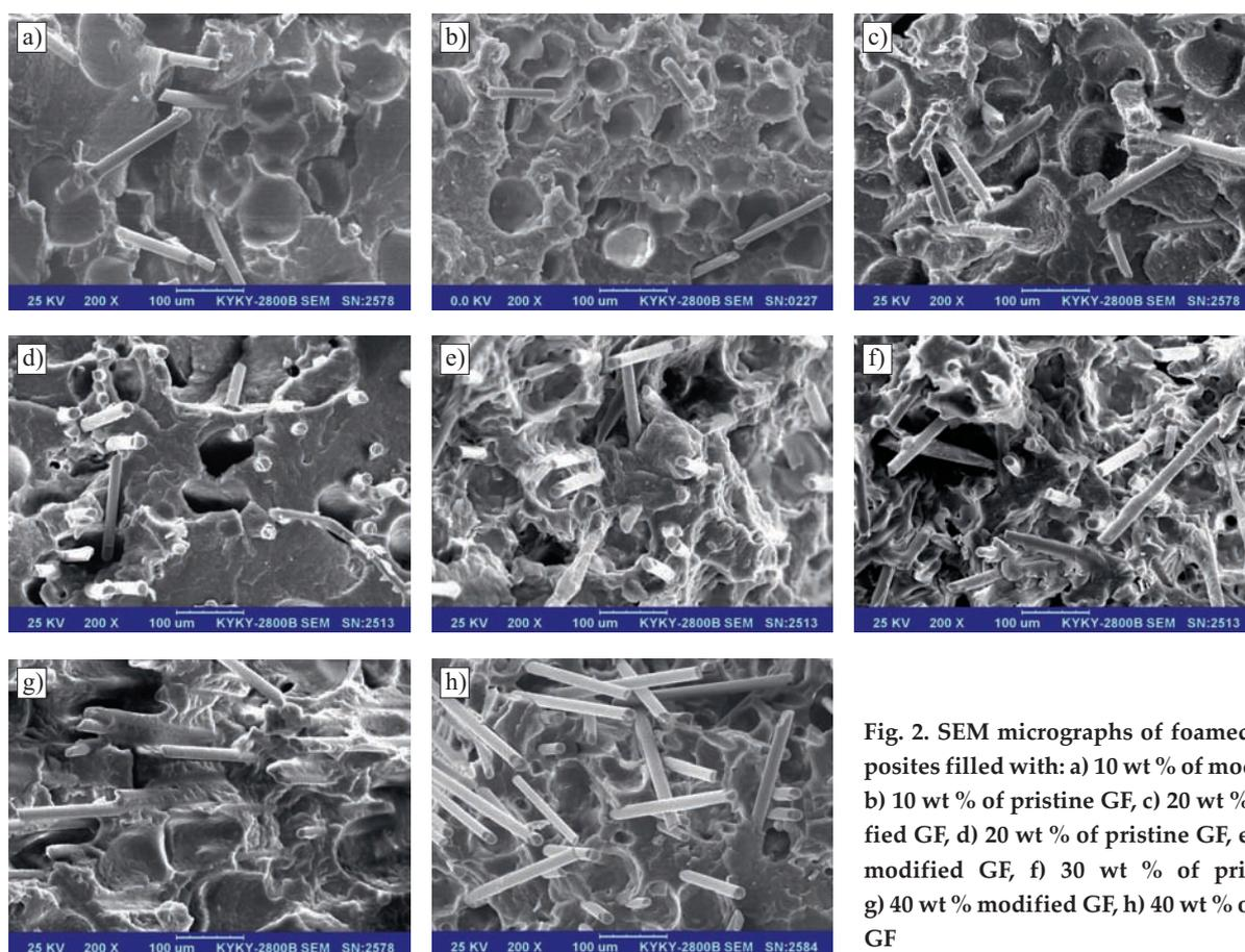
Fig. 2. SEM micrographs of foamed PP composites filled with: a) 10 wt % of modified GF, b) 10 wt % of pristine GF, c) 20 wt % of modified GF, d) 20 wt % of pristine GF, e) 30 wt % modified GF, f) 30 wt % of pristine GF, g) 40 wt % modified GF, h) 40 wt % of pristine GF
