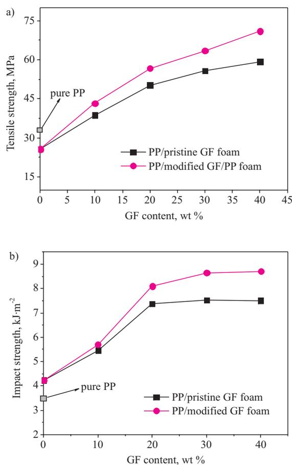
Fig. 1. The influence of pristine and modified GF content in microcellular foamed PP/GF composites on: a) tensile strength, b) impact strength
