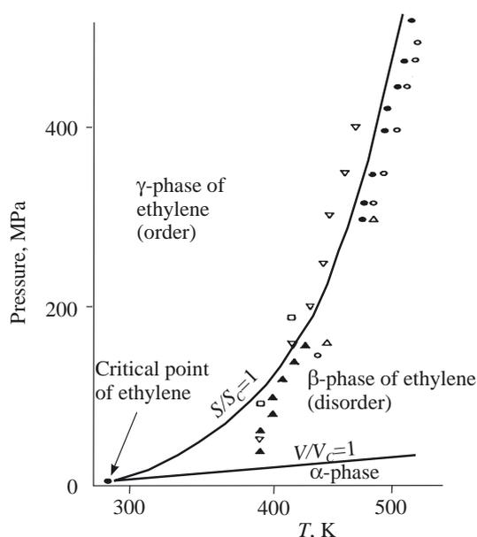
Fig. 10. Phase transitions in compressed ethylene gas (solid line  $S/S_c = 1$ ) and in compressed polyethylene (points) [23]
