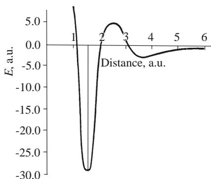
Fig. 5. Potential energy  $E$  as a function of the distance between an adsorbate molecule from the surface, i.e. transition from the physical to the chemisorption [11] (arbitrary units for  $E$  and distance)
