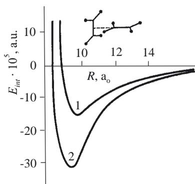
Fig. 4. Curves of potential energy  $E_{int}$  as a function of distance  $R$  between two ethylene molecules [10] (the curves 1 and 2 are theoretically calculated by two different methods);  $E_{int}$  is in atomic units (A.U.), where  $A.U. = 2.6253 \cdot 10^6$  kJ/mole;  $R$  is in  $a_0$  units, where  $a_0 = 5.2918 \cdot 10^{-7}$  cm
