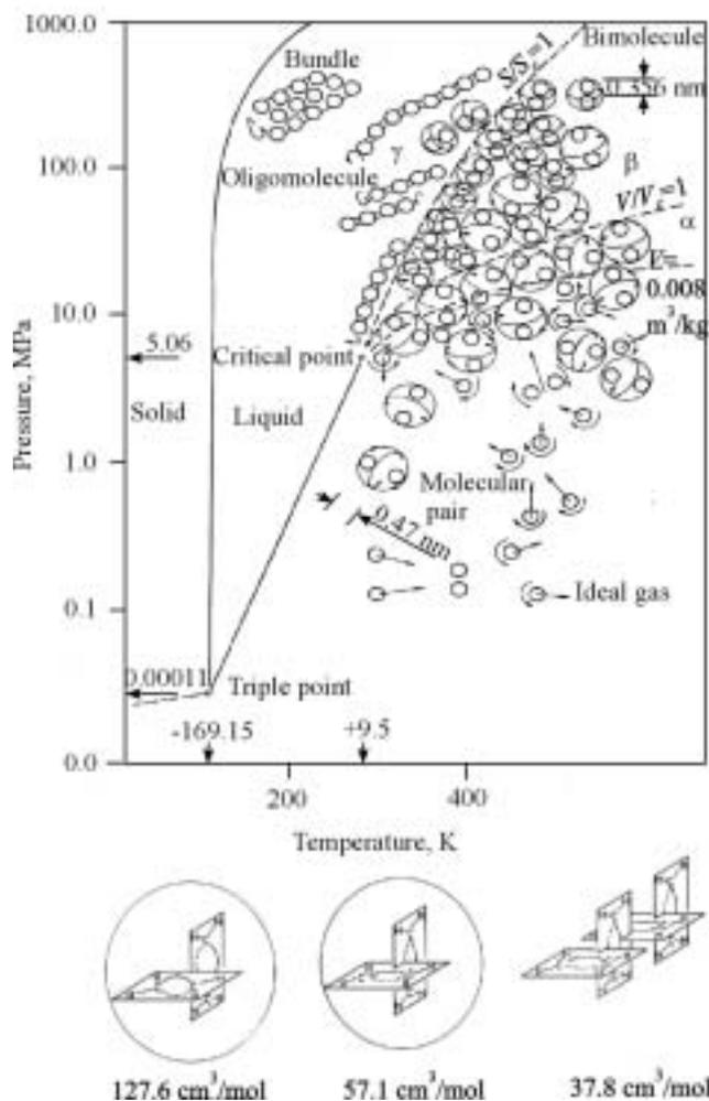
Fig. 9. Phase state (top) and supra-molecular species (bottom) and their volumes (empirical values) of compressed ethylene gas (molecular pair, bimolecule and oligomolecule, respectively) [18—23]
