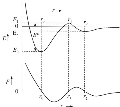
Fig. 2. Potential energy diagram that illustrates the dependence of the potential energy  $E$  on the distance of separation  $r$  of two atoms [8]. The bottom diagram is the corresponding force  $F$  acting between the atoms, obtained from the relation  $F = -\partial E/\partial r$
