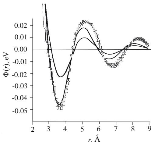
Fig. 3. Change of potential energy  $\phi(r)$  as a function of the distance  $r$  between two atoms of liquid sodium [9] (solid lines are the theoretical calculations; the points are the experimental values)
