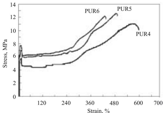
Fig. 10. Stress — strain curves of HMCD-polyurethane elastomers
