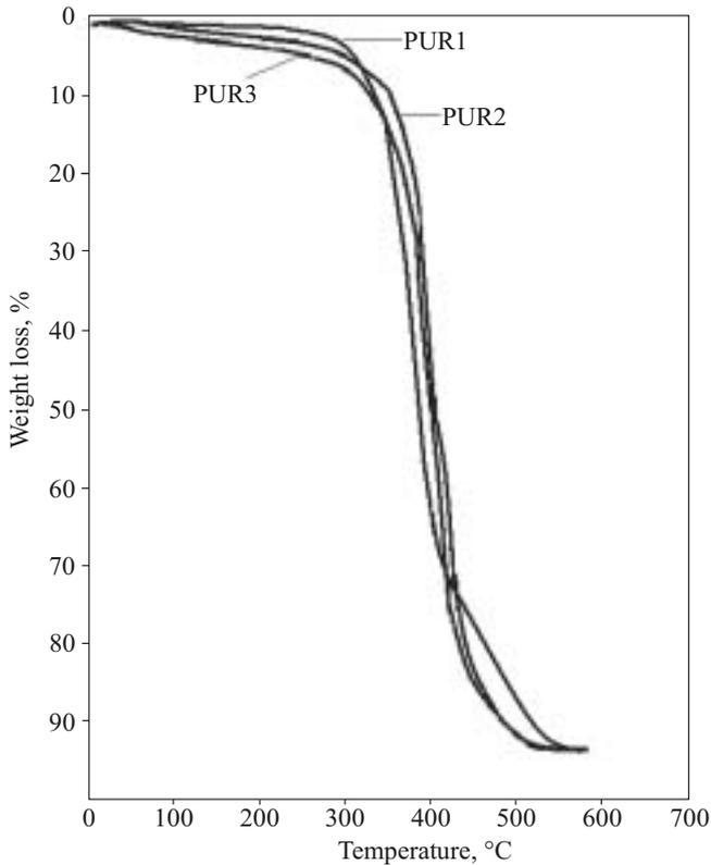
Fig. 3. TGA curves of CHD-based polyurethane elastomers
