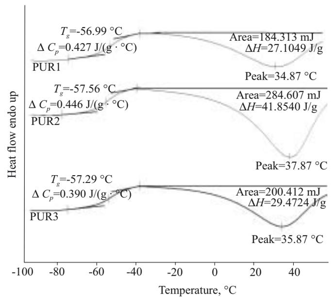
Fig. 5. DSC plots of CHD-polyurethane samples
