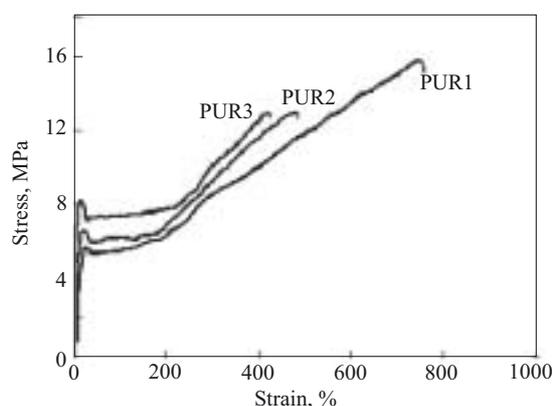
Fig. 9. Stress-strain curves of CHD-polyurethane elastomers
