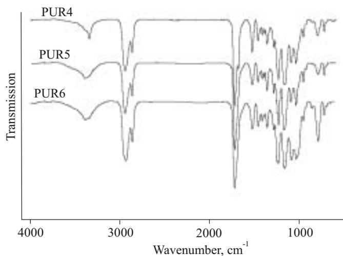
Fig. 2. FTIR spectra of polyurethane elastomers synthesized with HMCD as chain extender
