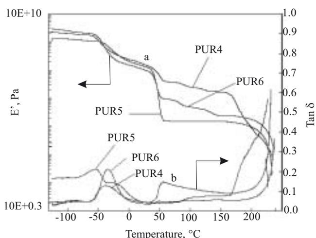
Fig. 8. Typical DMA spectra of the polyurethane samples with HMCD: a) storage modulus —  $E'$ , b) damping —  $\tan \delta$
