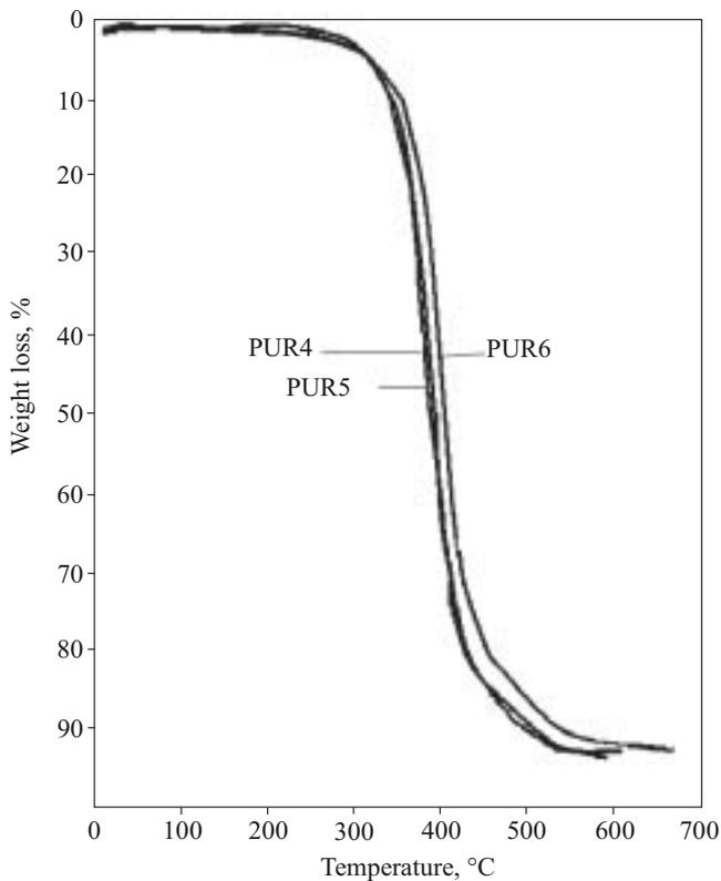
Fig. 4. TGA curves of HMCD-based polyurethane elastomers
