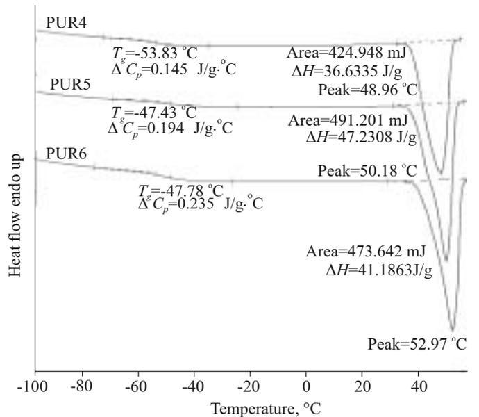
Fig. 6. DSC scan plots of HMCD-polyurethane samples
