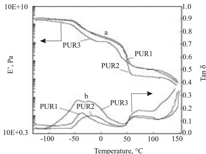
Fig. 7. Typical DMA spectra of the polyurethane samples with CHD: a) storage modulus —  $E'$ , b) damping —  $\tan \delta$
