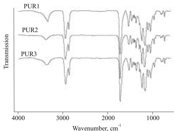
Fig. 1. FTIR spectra of polyurethane elastomers synthesized with CHD as chain extender
