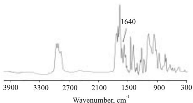
Fig. 4. FTIR spectrum of polymethacrylate resin **4a**
