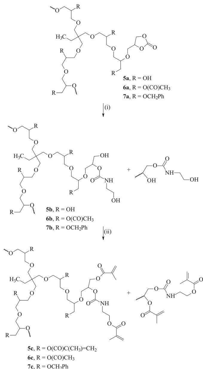
Scheme B. Synthesis of multimethacrylate resins containing urethane linkages: (i) 2-ethanolamine, 90 °C; (ii) methacrylic anhydride, 4-dimethylaminopyridine, DMF, room temperature
