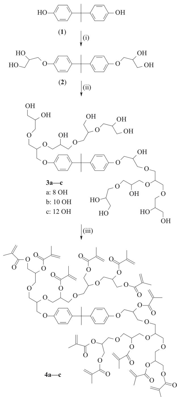
*Scheme A. The synthesis of bisphenol A based hyperbranched polyethers: (i) glycerol carbonate,  $K_2CO_3$ , 160 °C; (ii) glycidol, potassium, 90 °C; (iii) methacryloyl chloride, DMF, triethylamine, room temperature*
