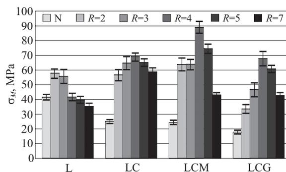
Fig. 6. Effect of the blow-up ratio ( $R$ ) of the studied films on tensile strength ( $\sigma_M$ )
