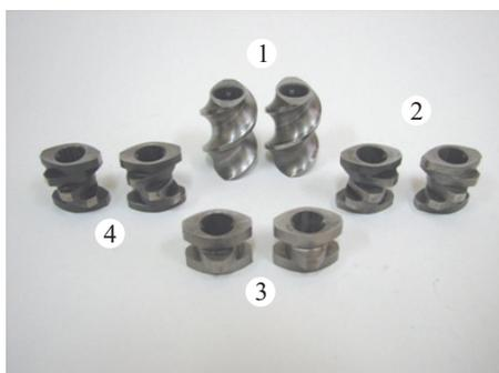
Fig. 1. Exchangeable screw segments: transporting (1), suppressing (2), neutral (3), and kneading (4)
