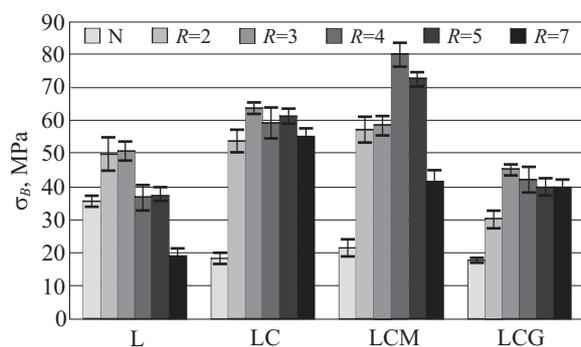
Fig. 7. Effect of the blow-up ratio ( $R$ ) of the studied films on tensile stress at break ( $\sigma_B$ )
