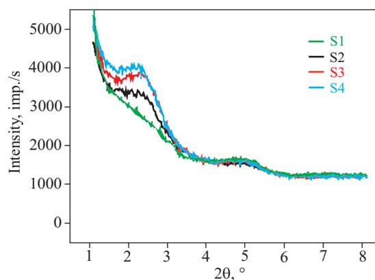
Fig. 4. XRD patterns of the LCG nanocomposite prepared using the S1, S2, S3, and S4 screws
