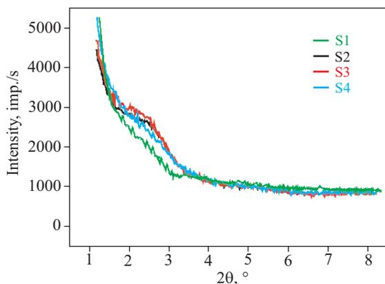
Fig. 2. XRD patterns of the LC nanocomposite prepared using the S1, S2, S3, and S4 screws
