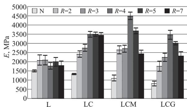
Fig. 5. Effect of the blow-up ratio ( $R$ ) of the studied films on longitudinal modulus of elasticity ( $E$ )
