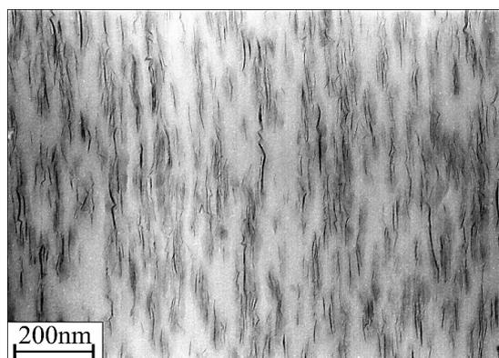
Fig. 9. TEM image of LC film with the blow-up ratio  $R = 4$
