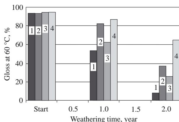
Fig. 3. Gloss at natural weathering (Florida 45° South) of epoxy acrylic silicone hybrid coatings based on epoxy functional polysiloxane and acidic functional acrylic resin (3 — not washed, 4 — washed) in comparison with polyurethane (1 — not washed, 2 — washed)
