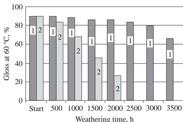
Fig. 2. Artificial QUV-A (1) and QUV-B (2) weathering of epoxy acrylic amine silicone hybrid coating based on glycidoxy functional acrylic resin and amino functional polysiloxane
