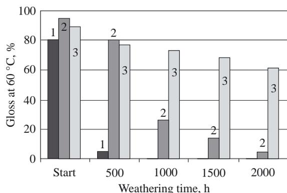
Fig. 1. Artificial QUV-B weathering of epoxyamine silicone hybrid coating (3) in comparison with control samples: epoxy amine (1) and polyurethane (2)
