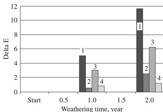
Fig. 4. Colour change (delta E) at natural weathering (Florida 45° South) of epoxy acrylic silicone hybrid coatings based on epoxy functional polysiloxane and acidic functional acrylic resin (3 — not washed, 4 — washed) in comparison with polyurethane (1 — not washed, 2 — washed)
