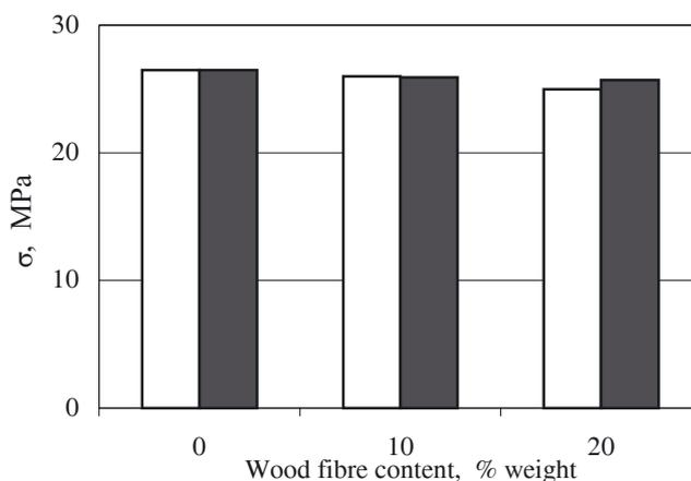
Fig. 2. Comparison of tensile strength ( $\sigma_M$ ) of the composites of recycled PP with different content and type of wood flour; □ — CB 120, ■ — BK 40/90
