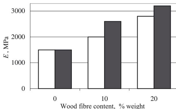
Fig. 1. Comparison of tensile modulus ( $E$ ) of the composites of recycled PP with different content and type of wood flour; □ — CB 120, ■ — BK 40/90
