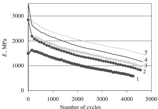
Fig. 6. Comparison of elasticity modulus ( $E$ ) under cyclic loading of PP composites with two types of wood flour; for symbols — see Fig. 5
