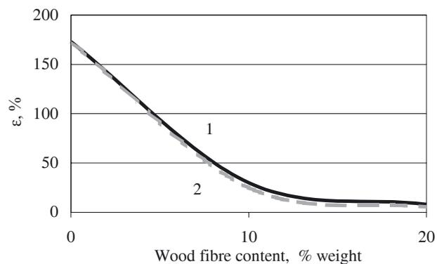
Fig. 3. Comparison of elongation at break ( $\epsilon$ ) of the composites of recycled PP with different content and type of wood flour, 1 — PP with CB 120, 2 — PP with BK 40/90
