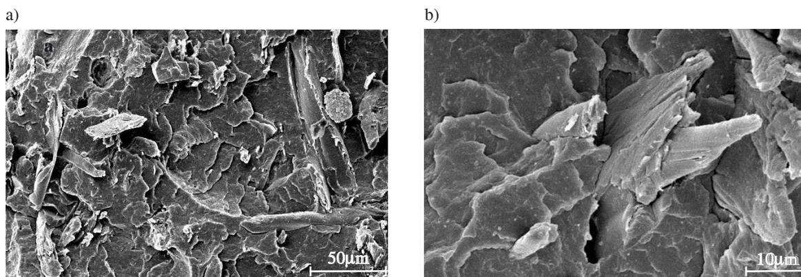
Fig. 10. SEM images of PP composites filled with 20 wt. % of wood flour (CB 120): a) magnification 500 times, b) magnification 2000 times
